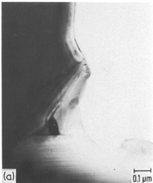
Figure 13 STEM micrographs of a triple-point region of SSiC I: (a) bright-field; (b) dark-field.
