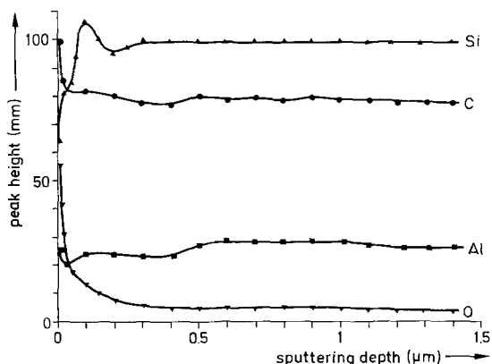
Figure 4 AES depth analysis of a selected Al-rich area in the fracture surface of SSiC I.
